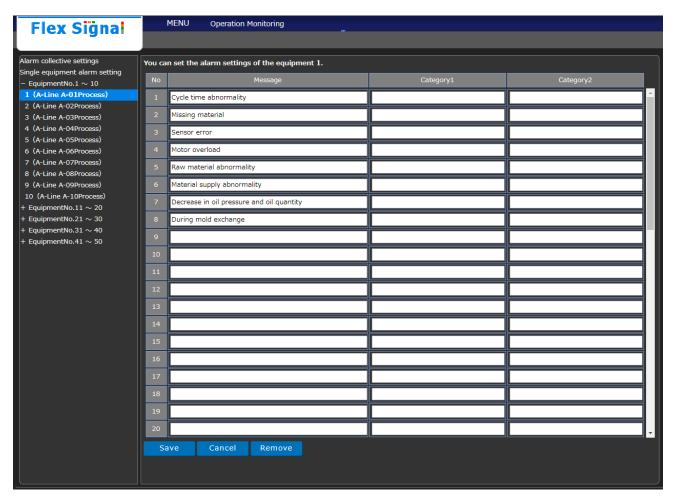
Figure 13: Single equipment alarm setting screen
