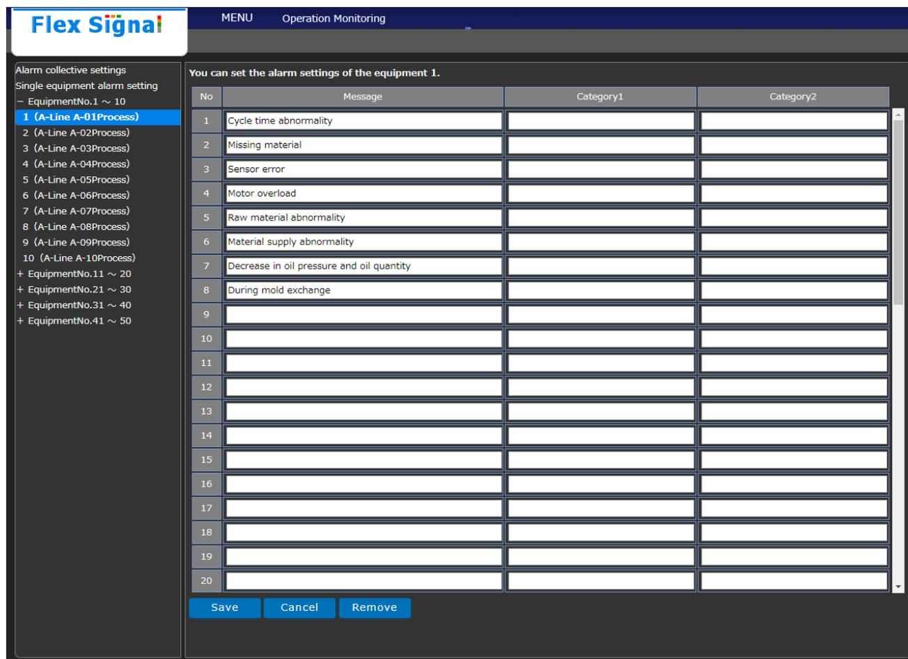
Figure 13: Single equipment alarm setting screen
