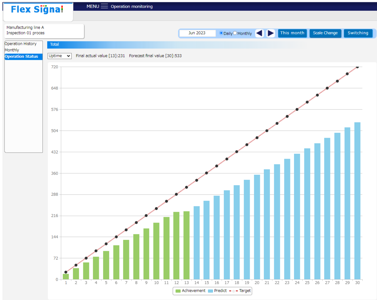
Figure 11: Operating state monitor screen (Graph of operating time and production volume)
